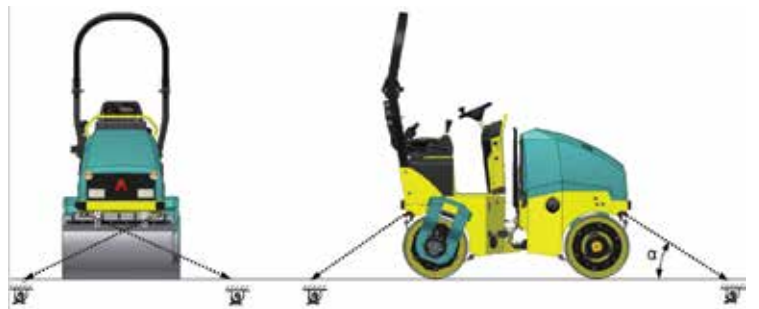
4 large tie down points for safe fixing onto trailer / truck
