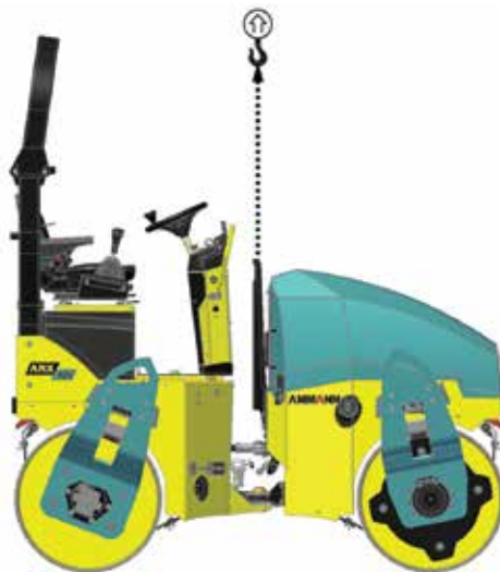
Central lifting point on ARX1(standard) ARX2 (option)
